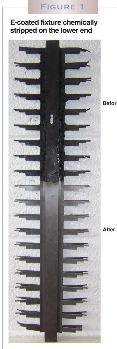
**FIGURE 2****An e-coated rack chemically stripped**
